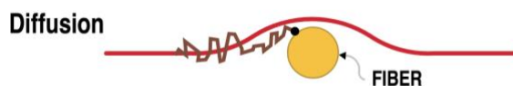
Figure 2. The red line indicates air moving around a filter fibre (yellow circle). The black dot indicates a particle. [9]
